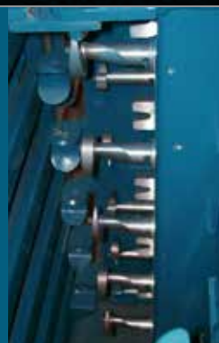
Maren's unique 100% gear driven twister maintains perfect twister timing.
