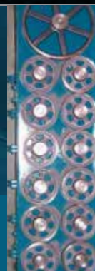
Maren's unique 100% gear driven twister maintains perfect twister timing.
